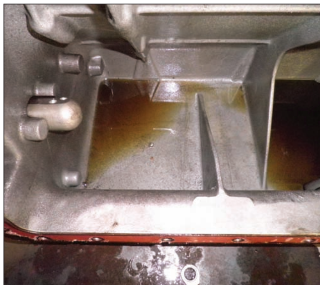
Visible chunks of metal in the sump of the disassembled engine
