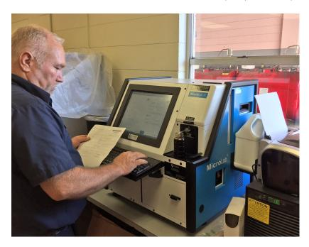
All the user has to do is insert a sample, input some basic information about the oil and equipment and the instrument performs up to four different types of analyses. These analyses provide a complete picture of the oil and powertrain condition.
